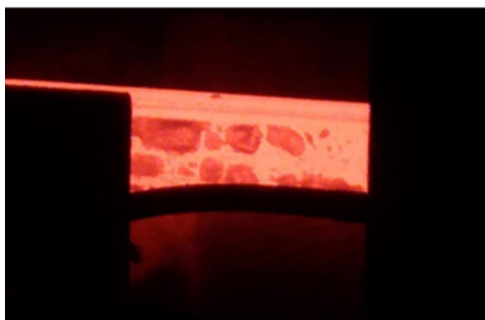
Fig.13. Incomplete descaling of billet and rolls to form seams.
